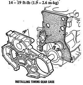
4. Trim off the protruding parts of the gasket between the cylinder block and the timing gear case.
