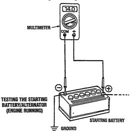
3. Turn off the engine. Inspect all wiring and connections. Ensure that the battery terminals and the engine ground connections are tight and clean.
