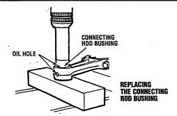
5. After pressing the bushing in, correct its inner diameter with a spiral expansion reamer so that the clearance will be within the standard value.
