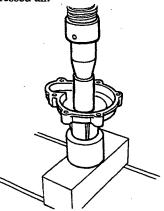
6. Press the impeller onto the shaft/bearing.
