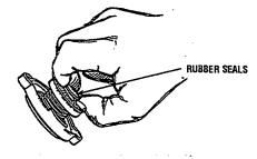
CHECKING THE PRESSURE CAP
