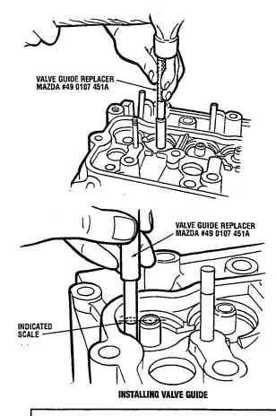
**CAUTION:** When the valve guide is replaced, recheck the clearance between the valve and the valve guide.
