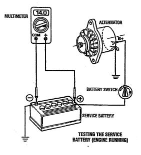
**A CAUTION:** To avoid damaging the alternator diodes, do not use a high voltage tester (i.e. a megger) when performing tests on the alternator charging circuit.
