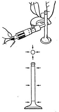
CHECKING VALVE STEM OIL CLEARANCE
