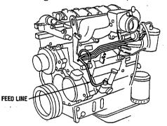
INSTALLING FUEL FEED LINE
