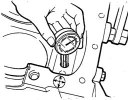
MEASURING INNER DIAMETER OF TAPPET GUIDE
