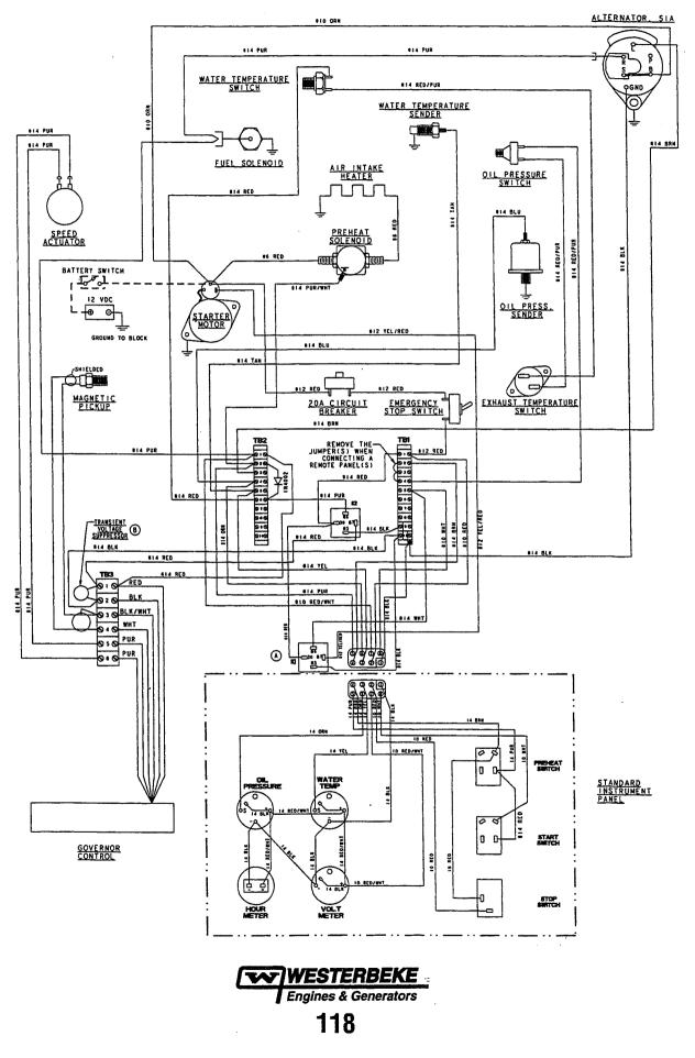
**32 KW BEDA GENERATOR** WIRING SCHEMATIC #040425 (TWO RELAYS)
