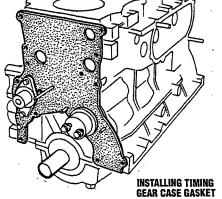
3. Install the timing gear case. Timing gear case tightening torque:
