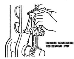
Connecting rod torsion limit: 0.002 in (0.05 mm) per 1.97 in (50 mm)
