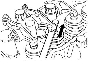
CHECKING THE VALVE CLEARANCE
