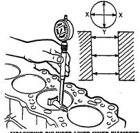
MEASURING CYLINDER LINER INNER DIAMETER
