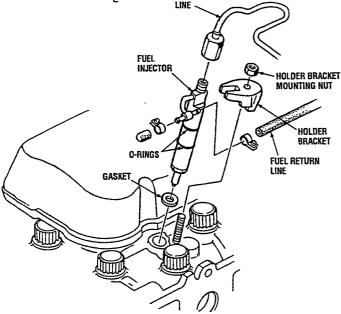
**REMOVING THE FUEL INJECTORS**
