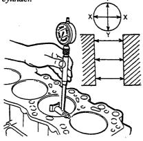
MEASURING CYLINDER INNER DIAMETER
