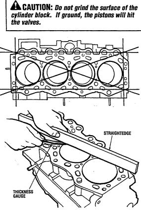
MEASURING CYLINDER BLOCK DISTORTION
