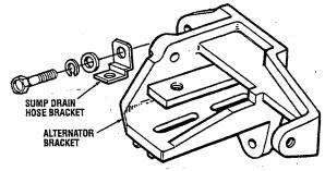
INSTALLING ALTERNATOR BRACKET
