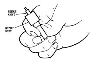
CHECKING THE NOZZLE BODY AND NEEDLE VALVE
