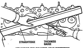
MEASURING THE CYLINDER HEAD DISTORTION
