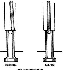
INSERTING PUSH RODS
