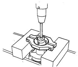
2. Press out the water pump impeller and shaft/bearing using the water pump impeller support block (Mazda #49 0823 146) and a press.
