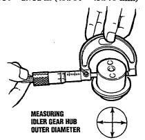
c. Calculate the oil clearance by subtracting the outer diameter of the idler gear hub from the inner diameter of the idler gear. If the clearance exceeds the specified limit, replace the idler gear bushing and the idler gear hub.
