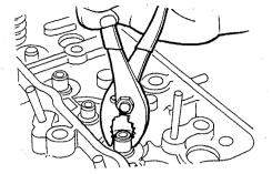
c. When removing the valves, make sure each valve is marked so it can be returned to its original position, if reused.
