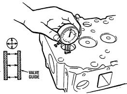
MEASURING INNER DIAMETER OF VALVE GUIDE
