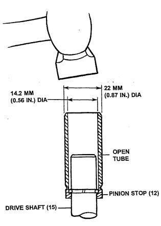
FIGURE 8. REMOVING PINION STOP
