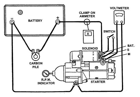
FIGURE 2. STARTER NO-LOAD TEST HOOK-UP
