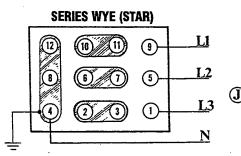
L - L - 450 VAC 3Ø 60Hz L - N - 265 VAC 1Ø 60 Hz L - L- 380 VAC 3Ø 50Hz L - N - 230 VAC 1Ø 50Hz
