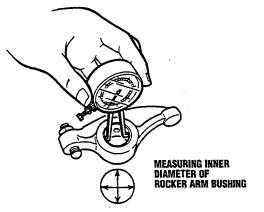
c. Calculate the oil clearance by subtracting the outer diameter of the rocker shaft from the inner diameter of the rocker arm bushing. If the oil clearance is outside the specified limits, replace the rocker arm bushing or the rocker arm shaft.
