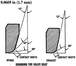
3. To seat the valves, apply a thin coating of engine oil mixed with a small amount of compound to the seat surface, then lightly tap while turning the valve.
