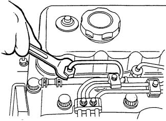
LOOSEN THE INJECTOR ENDS OF ALL FUEL LINES
