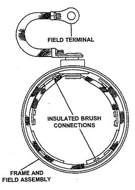
FIGURE 10. FRAME AND FIELD ASSEMBLY
