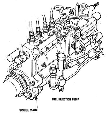
ALIGN THE SCRIBE MARK ON THE INJECTION PUMP FLANGE WITH THE SCRIBE MARK ON THE GEAR CASE, THIS WILL PLACE THE INJECTION PUMP IN PROPER TIMING WITH THE ENGINE.
