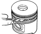
CHECKING PISTON RING AND GROOVE CLEARANCE
