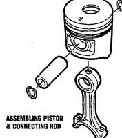
f. Check to make sure the connecting rod can be easily moved.
