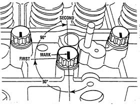
MARKING THE CYLINDER HEAD BOLTS
