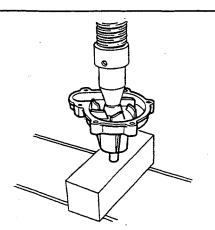
7. Press in the water pump flange using a pipe of the specified size.
