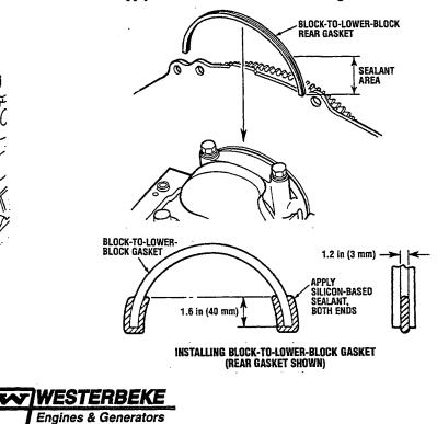
2. Install the right and left block-to-lower-block gaskets onto the cylinder block and then install the lower block.
