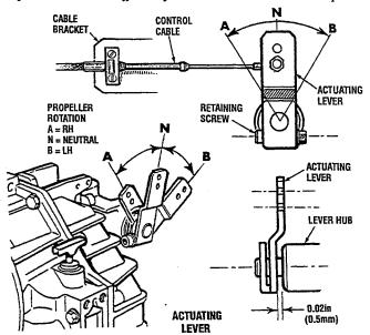
A greater amount of actuating lever travel is in no way detrimental and is recommended. However, if the lever travel is shorter, proper clutch engagement might be impeded which, in turn, would mean premature wear, excessive heat generation and clutch plate failure. This would be indicated by slow clutch engagement or no engagement at all (see *CONTROL CABLES* under *TRANSMISSION TROUBLESHOOTING*)
