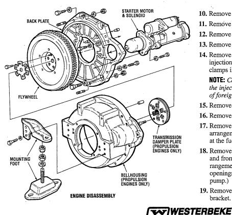
8. Remove the transmission damper plate (propulsion engines only).
