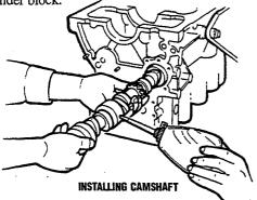
2. Install the camshaft retaining plate with the flush side facing the cylinder block.
