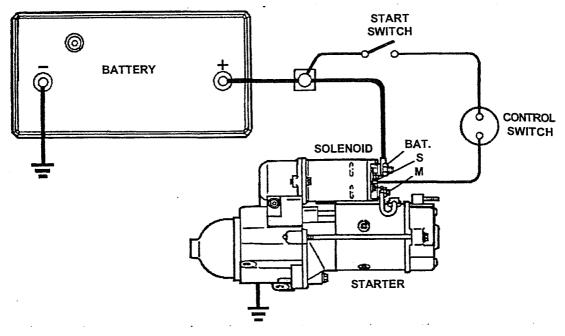
FIGURE 1. STARTER WIRING CIRCUIT
