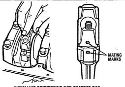
INSTALLING CONNECTING ROD BEARING CAP
