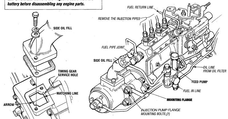
Remove the gear case side oil filter neck. This will expose the gear cover service hole.
