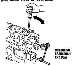
7. If the end play is not within the standard range, select a suitable thrust washer.
