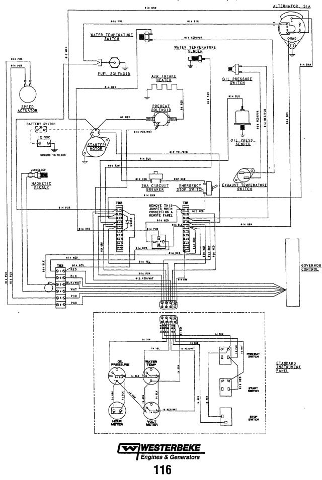
**32 KW BEDA GENERATOR** WIRING SCHEMATIC #040425 (SINGLE RELAY)
