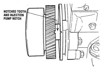
Align the notch in the injection pump with the notched tooth on the timing gear as shown above.
