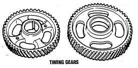
2. Measure the backlash of the idle gear and the other gears with a dial gauge. Gears not being measured should be kept disengaged.
