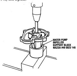
3. Tap out the seal using a pipe of the specified size.
