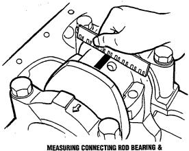
MEASURING CONNECTING ROD BEARING & CRANKSHAFT PIN JOURNAL OIL CLEARANCE
