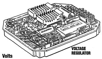
This potentiometer is used to adjust output voltage. At proper engine operating speed the output voltage should be held at  $\pm 1\%$  from a no-load condition to a full rated generator output and from power factor 1.0 - 0.8 with engine drive speed variations up to -6%.
