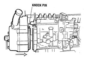
Position the injection pump so the knock pin on the timing gear case and its hole on the injection pump flange are aligned, then install the injection pump. Tighten the installation bolts to the specified torque. If the alignment is not correct, remove the injection pump and repeat the installation procedures.
