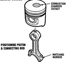
e. Assemble the piston and connecting rod with the piston pin and lock the snap rings so the pin won't come out.
