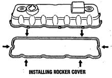
4. Put the rocker cover outer gasket on the rocker cover's cover and install.
