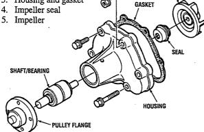
1. Press out the coolant pump pulley flange using a suitable puller and a press.
